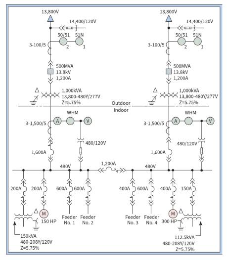
Fig. 4. Example of a typical one-line diagram.
