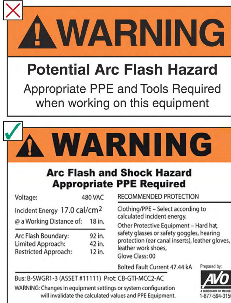
Fig. 2. Two examples of arc flash warning labels. The top label is inadequate, as it's missing a lot of crucial information.
