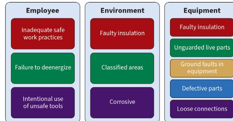
Fig. 1. Three key factors come into play with an arc flash event.
