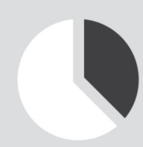
At 480 volts, arcing faults can be 40% of bolted faults
